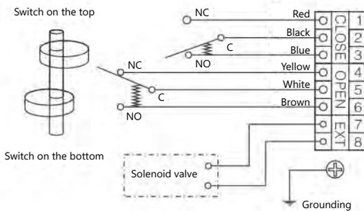
**Mechanical Switch (2SPDT)**
