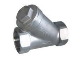
Y-type Female Strainer (CF8, CF8M, WCB) 1/4"~4" / 800PSI YS11F6N/800
