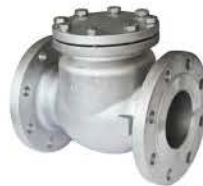
ANSI, JIS, DIN, GB Flanged Check Valve (CF8, CF8M) ANSI-1/2"~20" / 150LB~600LB JIS- DN15~500 / 10K~20K DIN- DN15~500 / PN16~63 GB- DN15~500 / PN16~63 CV44W6F/150
