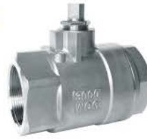
2PC Type Ball Valve Threaded Fire Safe (CF8, CF8M, WCB, Ti, Ni, LCC, LF2) 1/4"~2" / 3000PSI FBV12R6N/3000
