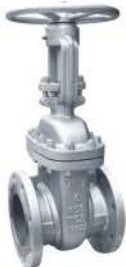
ANSI, JIS, DIN, GB Flanged Gate Valve (WCB) ANSI-1 1/2"~32" / 150LB~600LB JIS- DN40~500 / 10K~20K DIN- DN40~500 / PN16~63 GB- DN15~500 / PN16~63 GA40H5F/150
