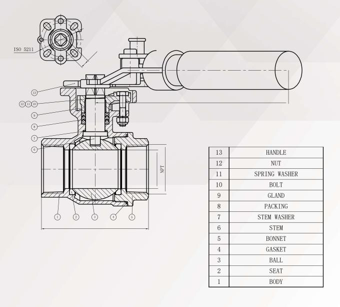
Refer to the diagram and parts list above for a detailed view of each component, assisting with installation, operation, and maintenance for optimal valve performance.
