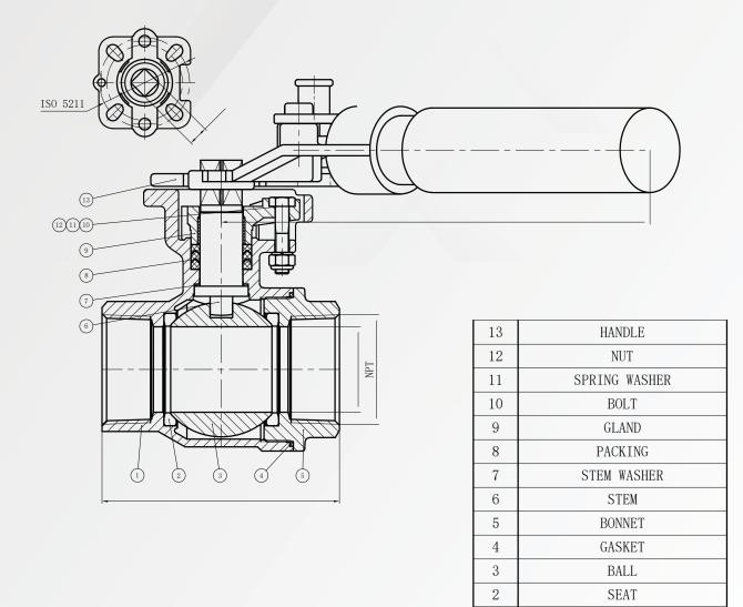
Refer to the diagram and parts list above for a detailed view of each component, assisting with installation, operation, and maintenance for optimal valve performance.
