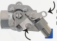
Engage locking mechanism onto bolt to lock valve
