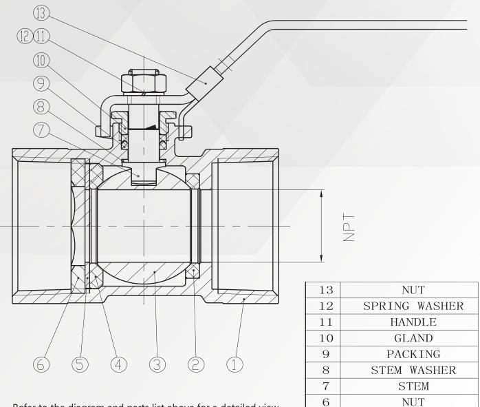
Refer to the diagram and parts list above for a detailed view of each component, assisting with installation, operation, and maintenance for optimal valve performance.
