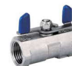
1PC Type Ball Valve With Internal Thread Butterfly Handle (CF8, CF8M, WCB) 1/4"~1" / 1000PSI
