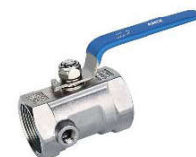
1PC Ball Valve With Test Hole (CF8, CF8M, WCB) 1/4"~4" / 1000PSI
