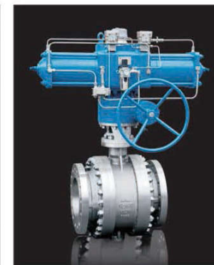
Pneumatic Flanged Ball Valve (CF8, CF8M, WCB, Ti, Ni) ANSI- 8"~28" / 150LB~300LB JIS- DN200~700 / 10K~20K DIN, BS- DN200~700 / PN16~63 GB- DN200~700 / PN16~63
