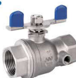
2PC Type With Test Hole Ball Valve With Internal Thread (CF8, CF8M, WCB) 1/4"~2" / 600PSI
